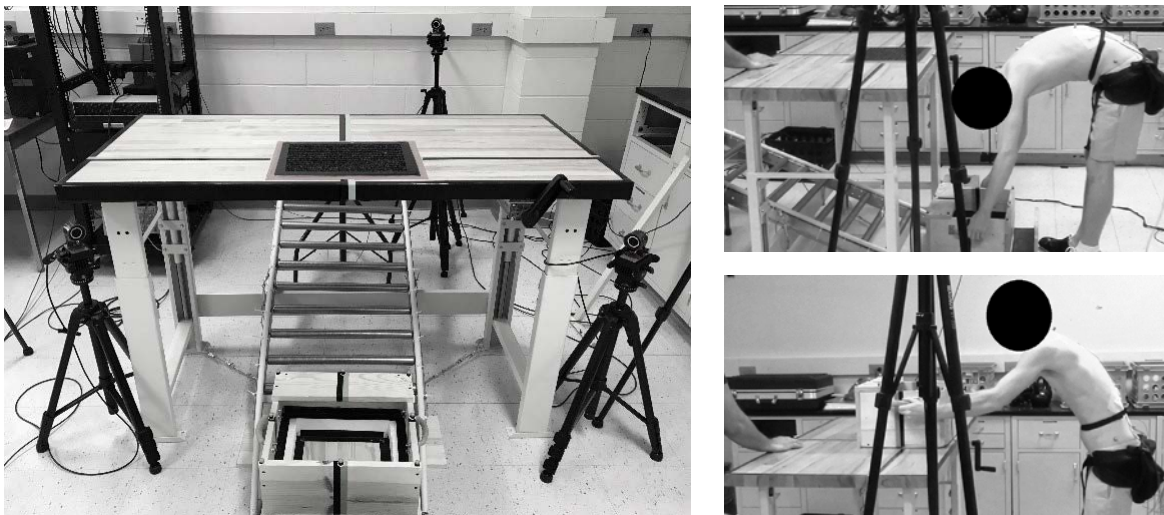
Figure 2.1 Task set-up with the roller conveyer ramp (left), and an example of a participant starting (top right) and ending (bottom right) a lifting cycle.
