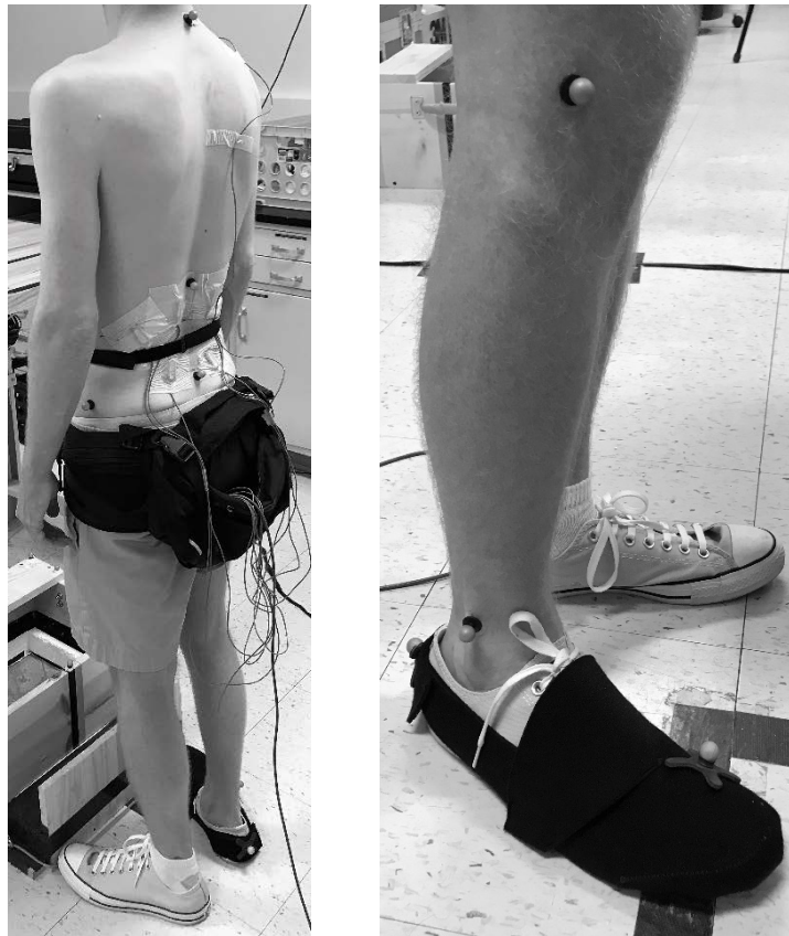
Figure 2.2 Marker configuration used in this study (for OMC data acquisition).
